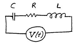
The above RLC circuit is underdamped (R <  $2\sqrt{\frac{L}{C}}$ ). It is driven by a time-varying external voltage given by:
