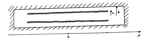
A current I flows in a long uniform air core solenoid of length £, radius a, and total number of turns N. The solenoid is centered in a long cylindrical cavity within a superconductor, as shown above. The cavity has radius b and length £', (For our purposes a superconductor is to be considered simply as a material which perfectly excludes magnetic fields, but note that surface currents will be induced in the superconductor.)
